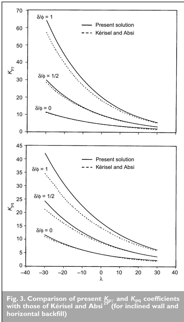
Fig. 3. Comparison of present  $K_{py}$  and  $K_{pq}$  coefficients with those of Kérisel and Absi<sup>29</sup> (for inclined wall and horizontal backfill)
