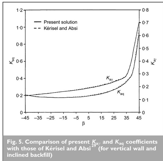
Fig. 5. Comparison of present  $K_{ay}$  and  $K_{aq}$  coefficients with those of Kérisel and Absi<sup>29</sup> (for vertical wall and inclined backfill)
