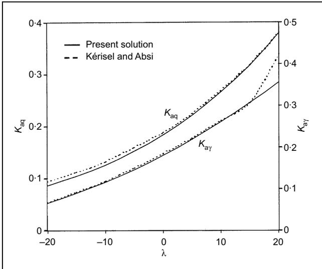
Fig. 6. Comparison of present  $K_{ay}$  and  $K_{aq}$  coefficients with those of Kérisel and Absi<sup>29</sup> (for inclined wall and horizontal backfill)
