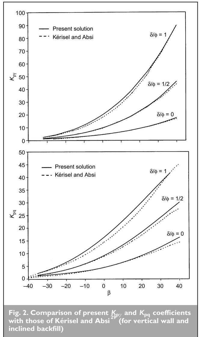
Fig. 2. Comparison of present  $K_{py}$  and  $K_{pq}$  coefficients with those of Kérisel and Absi<sup>29</sup> (for vertical wall and inclined backfill)
