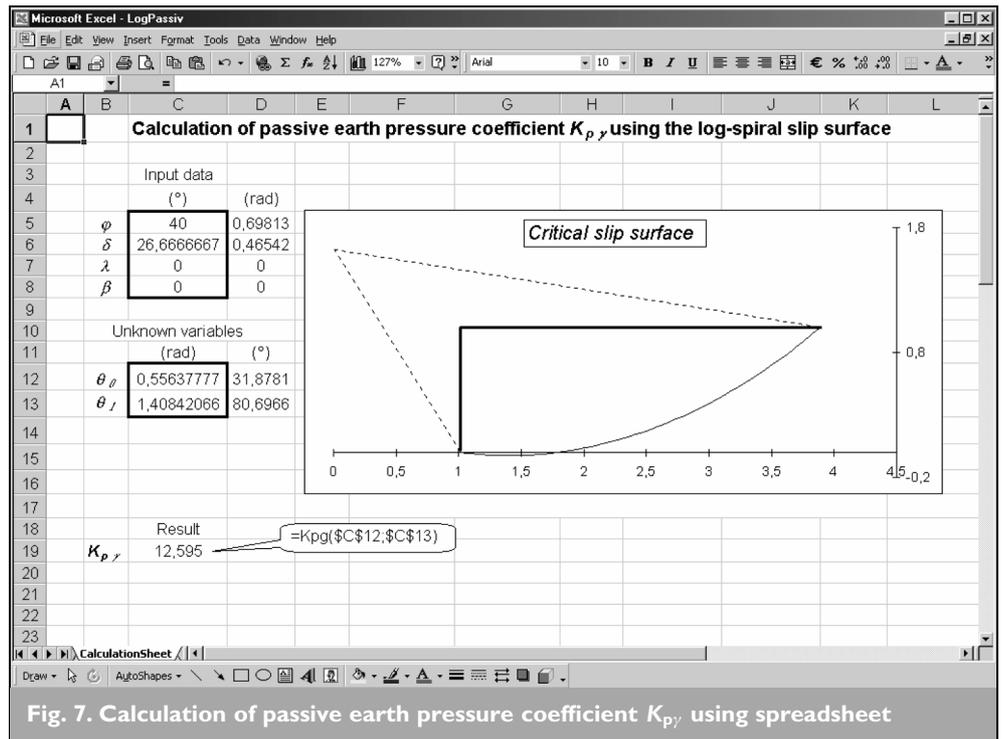
Fig. 7. Calculation of passive earth pressure coefficient  $K_{py}$  using spreadsheet
