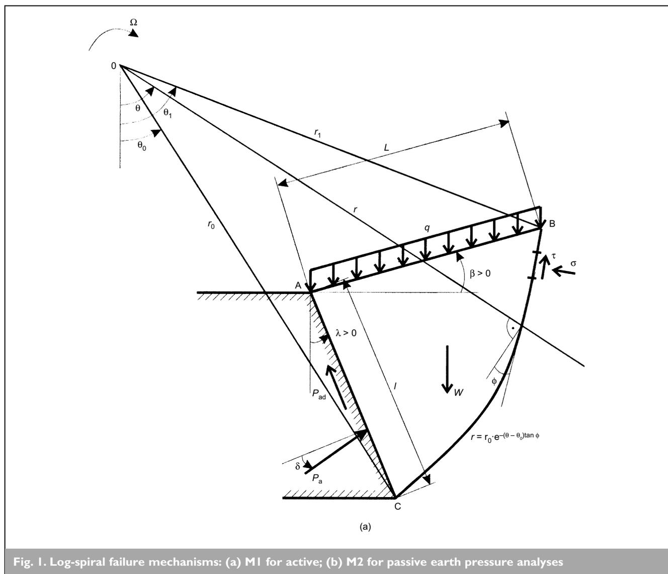
Fig. 1. Log-spiral failure mechanisms: (a) M1 for active; (b) M2 for passive earth pressure analyses
