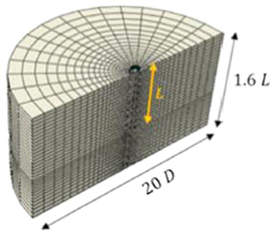
Fig. 15. Monopile foundation model [after El Haj et al. (2019)].
