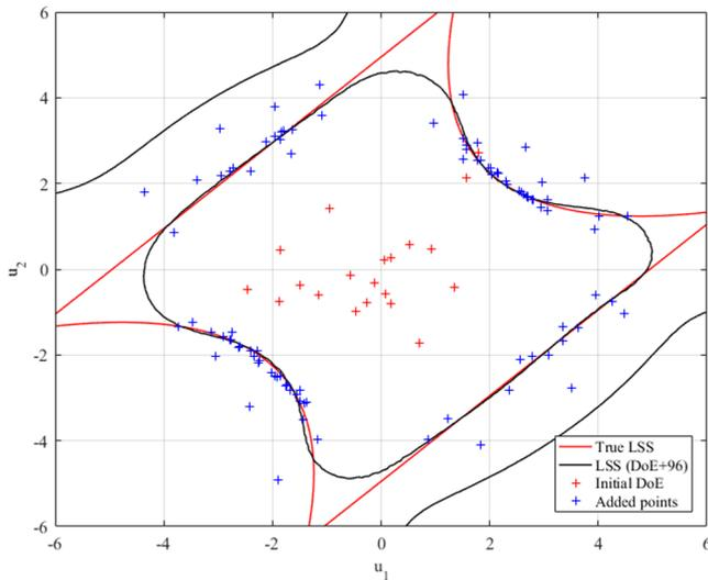
Fig. 10. Comparison between the LSS of the obtained metamodel (i.e. for 96 added points) and that of the true performance function.
