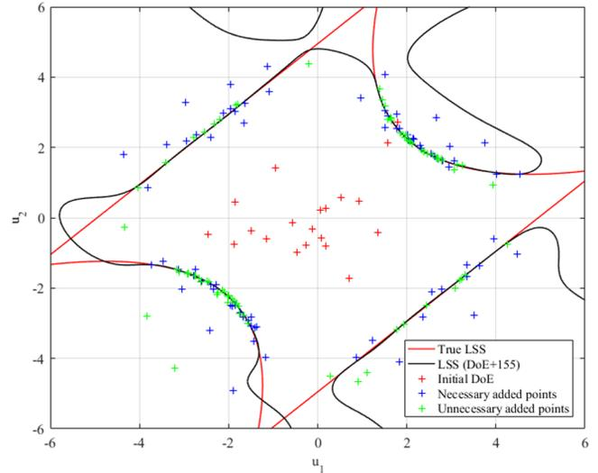
Fig. 11. Comparison between the LSS obtained by adopting the  $U$ -criterion (i.e. for 155 added points) and that of the true performance function.
