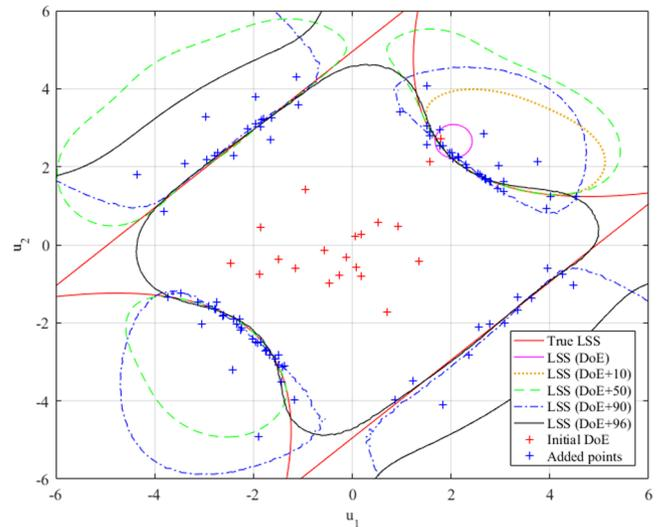
Fig. 8. Evolution of the limit state surface with the number of added points.
