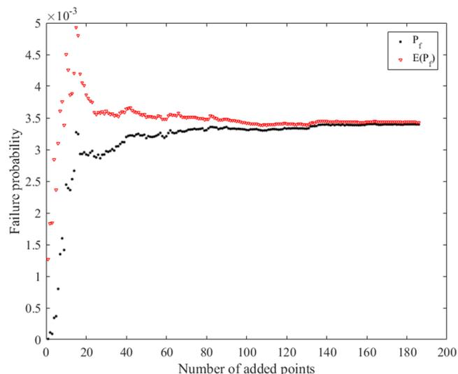
Fig. 18. Evolution of  $P_f$  and  $E(P_f)$  with the number of added points.
