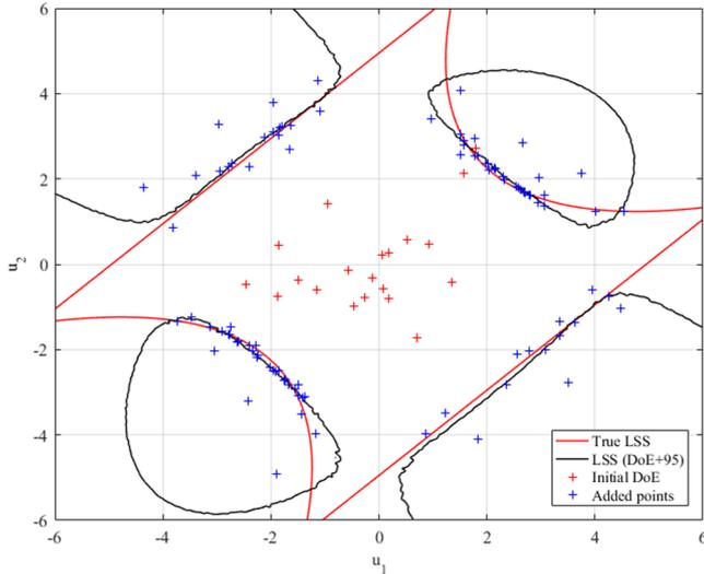
Fig. 9. Comparison between the LSS obtained one enrichment step before satisfying the proposed stopping criterion (i.e. for 95 added points) and that of the true performance function.
