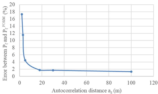
Fig. 20. Error with respect to FORM approximate method.
